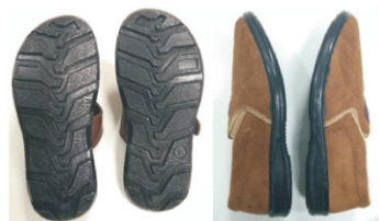
Figure.2 Complete footwear fabricated using the injection molded PU-nanofiller composite sole
